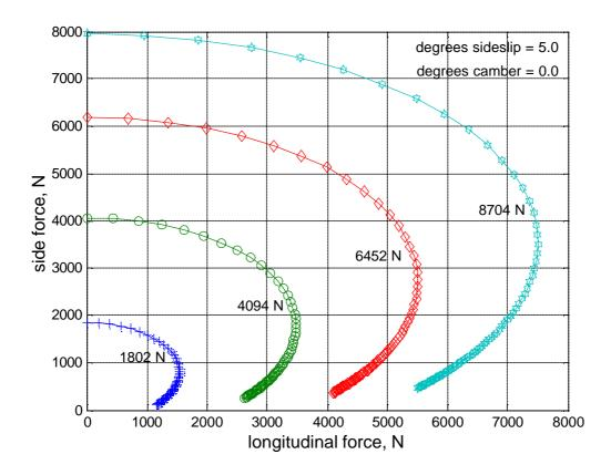
Fig. 14 Sideforce and braking force for 5 degrees sideslip angle and slip ratios from 0 to 1, reconstructed from the optimal parameter set
