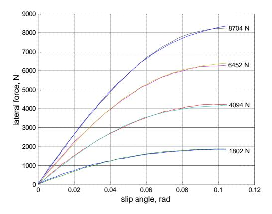
Fig. 12 Side forces for best fit E,  $b_4$ ,  $b_5$ ,  $b_{13}$  and  $b_{14}$  (see below for coefficients) with C constrained to be 1.65. Dotted lines show the fitted results
