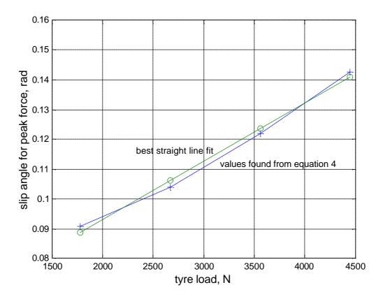
Fig. 2 Values of  $\boldsymbol{a}_p$  from solving (4) given B<sub>y</sub>, C and E for each of the four standard loads, and its straight line fit:  $\boldsymbol{a}_p = 0.000019463.F_z + 0.054238$
