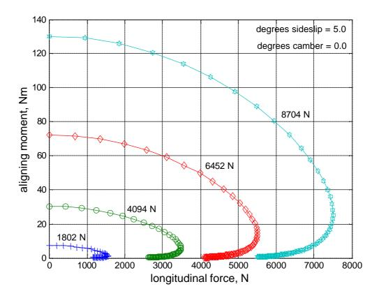
Fig. 15 Aligning moment for 5 degrees sideslip angle and slip ratios from 0 to 1, reconstructed from the optimal parameter set
