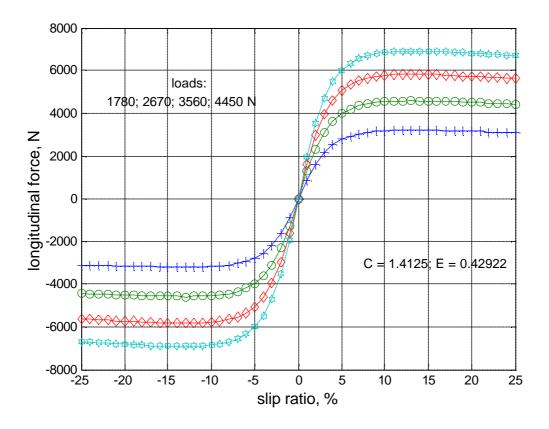
Fig. 6 Longitudinal forces as functions of slip ratio, using selected parameter values
