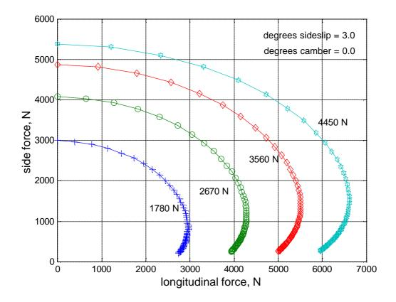
Fig. 7 Shear forces for 3 degrees sideslip and no camber, with longitudinal slip varying from 0 to 1 and four loads as shown
