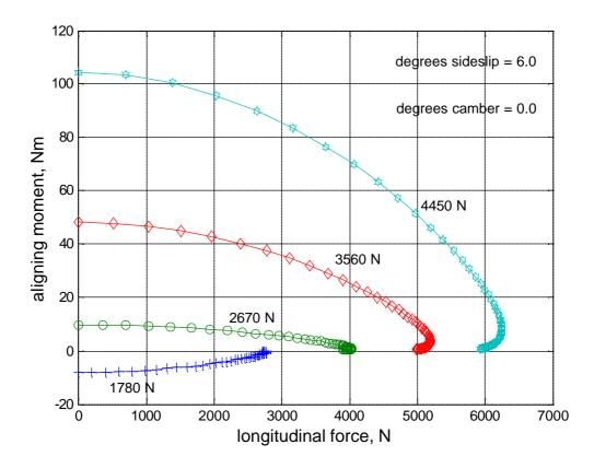
Fig. 10 Aligning moments for 6 degrees sideslip and no camber, with longitudinal slip varying from 0 to 1 and four loads as shown
