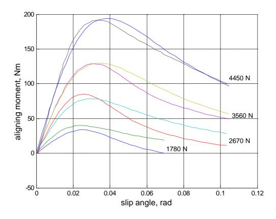
Fig. 4 Original (solid lines) and reconstructed (dotted lines) aligning moment data for Goodyear F1 front tyre,  $25.0 \times 9.0 - 13$  from reference [1], with C<sub>m</sub> = 2.099 and E<sub>m</sub> = -0.5929
