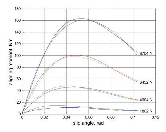
Fig. 13 Aligning moments for quadratic C and E values: Solid lines are for experimental results, while dotted lines are reconstructed
