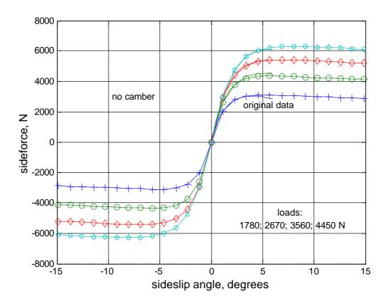
Fig. 3 Side forces as functions of sideslip angle using coefficients from fitting process and showing original data from reference [1]
