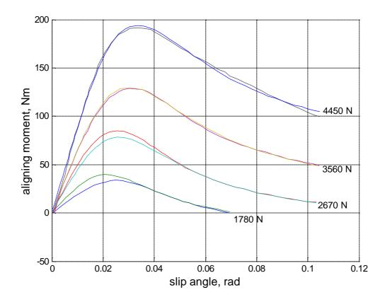
Fig. 5 Original (solid lines) and reconstructed (dotted lines) aligning moment data for Goodyear F1 front tyre, with  $C_m$  and  $E_m$  made quadratic functions of load
