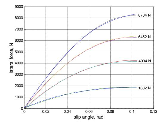
Fig. 11 Reconstructed side forces for best fit C, E,  $b_4$ ,  $b_5$ ,  $b_{13}$  and  $b_{14}$ . Solid lines show the experimental results from reference [1]; Dotted lines show the fitted results
