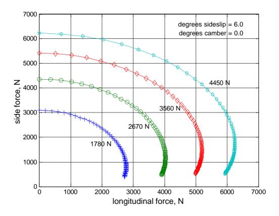
Fig. 9 Shear forces for 6 degrees sideslip and no camber, with longitudinal slip varying from zero to 1 and four loads as shown
