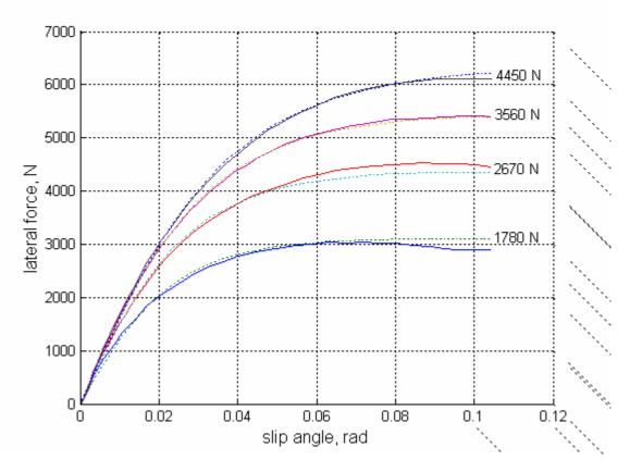
Fig. 1 Original (solid lines) and reconstructed (dotted lines) side force data for Goodyear F1 front tyre,  $25.0 \times 9.0 - 13$  from reference [1], with invariant C and E
