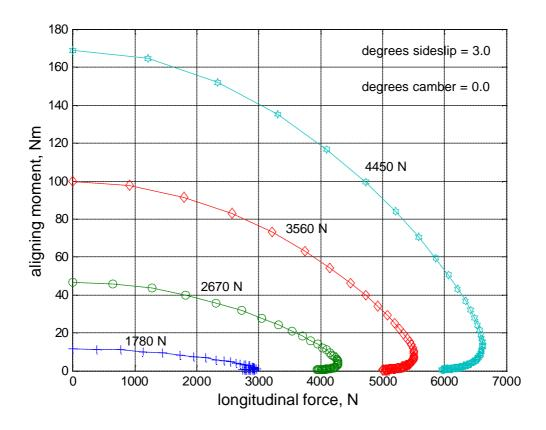
Fig. 8 Aligning moments for 3 degrees sideslip and no camber, with longitudinal slip varying from 0 to 1 and four loads as shown
