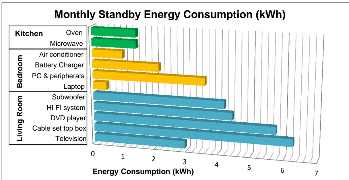
Figure 1: Bar Chart of the monthly standby energy consumption for each appliance
