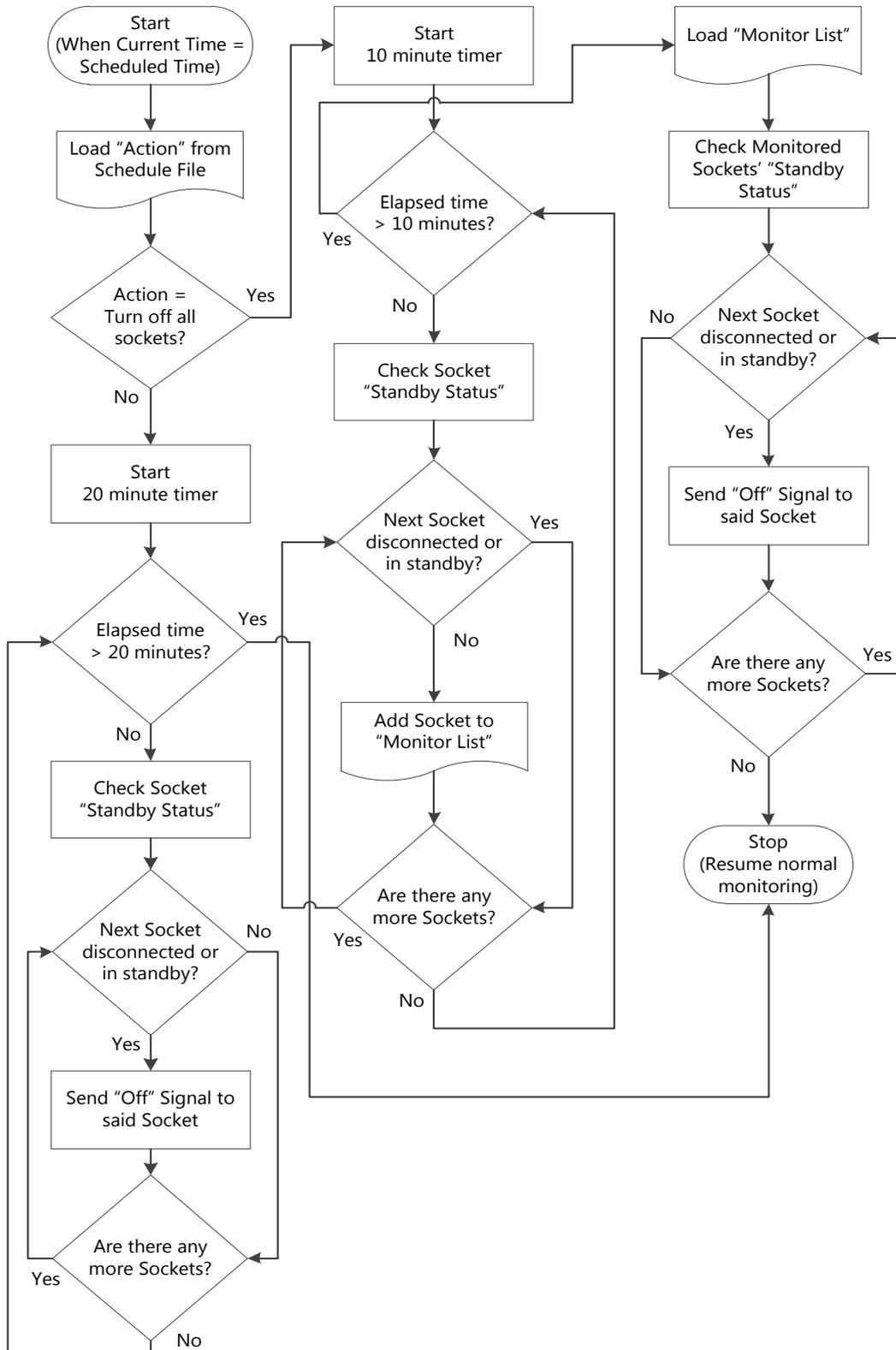
Figure 7. Schedule tolerance and timeout functions
