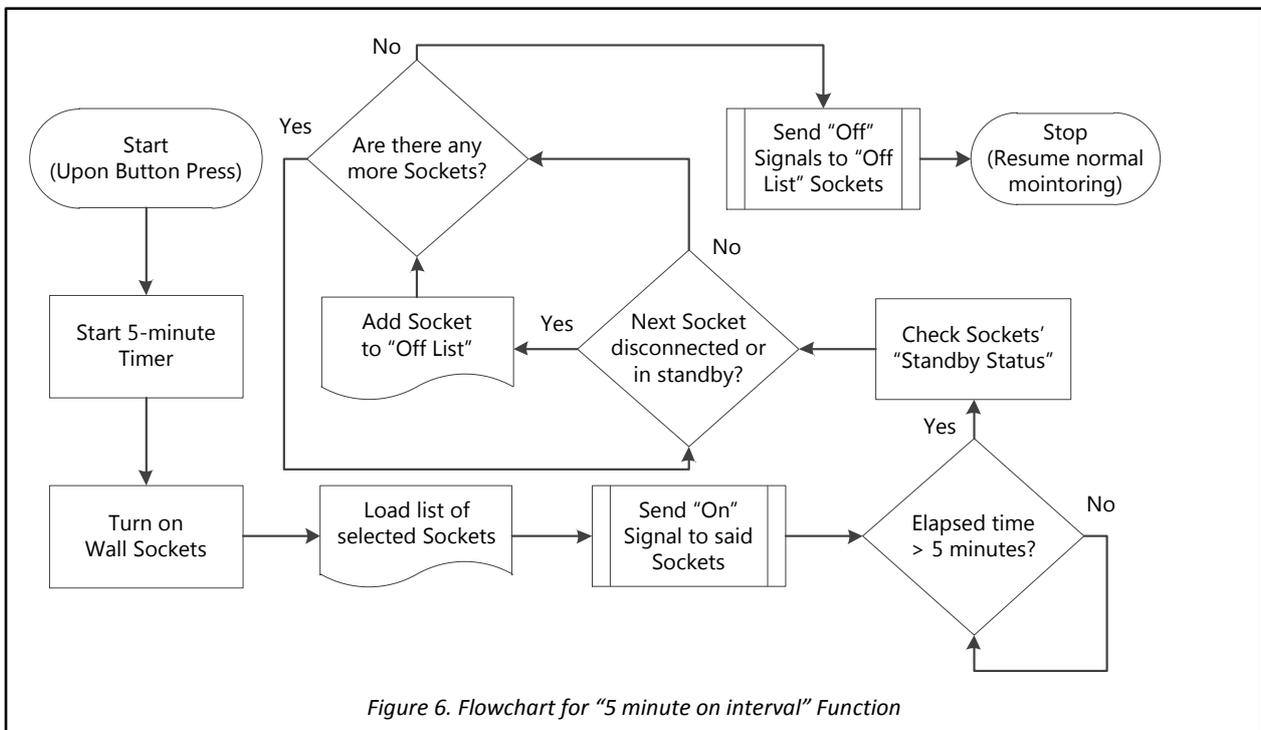
Figure 6. Flowchart for “5 minute on interval” Function
