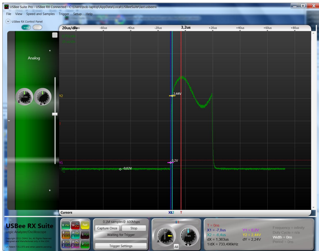
Figure 6: Shows arbitrary pulse waveform rise time and ripple
