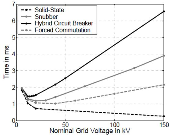
**Figure 4: Grid Voltage vs. Time [4]**
