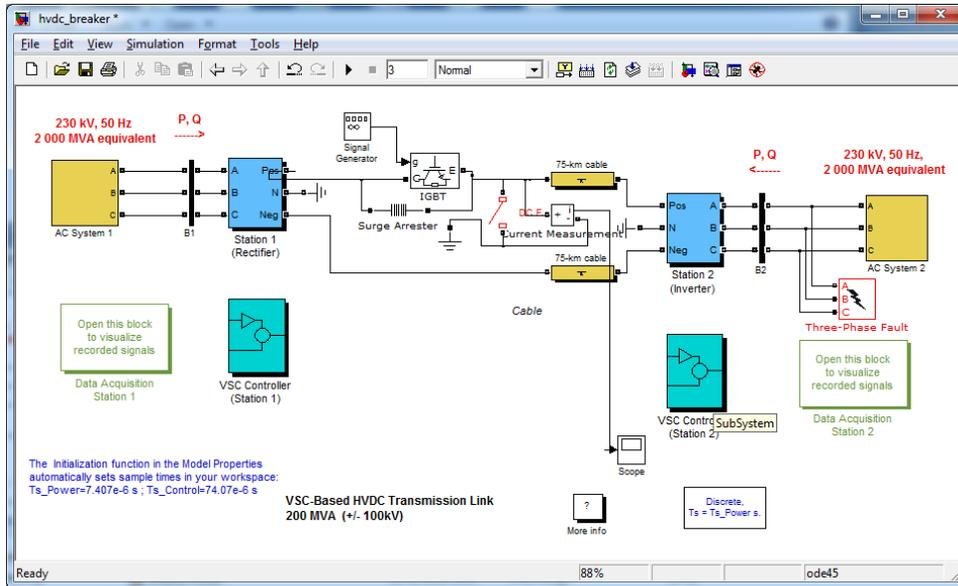
**Figure 7: HVDC MATLAB model**
