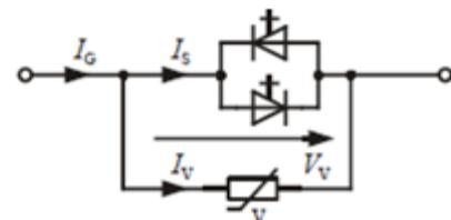
**Figure 3: Solid State Circuit Breaker [4]**
