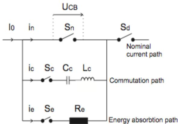
**Figure 2: Electromechanical Circuit Breaker [1]**
