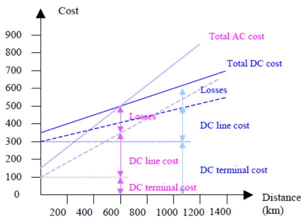
High Voltage Direct Current has been used for decades for transmission of power over long distances. The fact that capacitance in cables doesn't cause losses means that it makes up for drawbacks in the conversion process from AC, since HVDC conversion stations are more expensive than the AC ones. On the other hand, long distance HVDC lines cost in general less than the respective AC lines. As we can see from figure 1, above a certain distance HVDC transmission will have lower costs.
