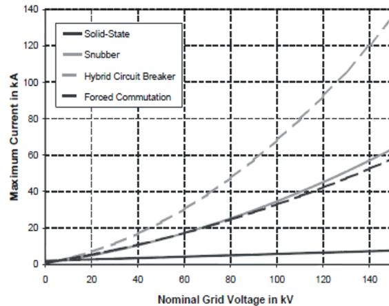
**Figure 5: Grid Voltage vs. Maximum Current [4]**
