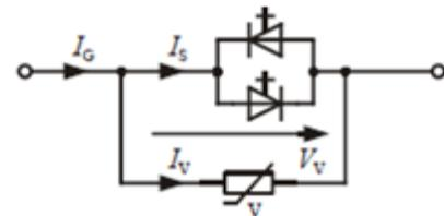
**Figure 3: Solid State Circuit Breaker [4]**
