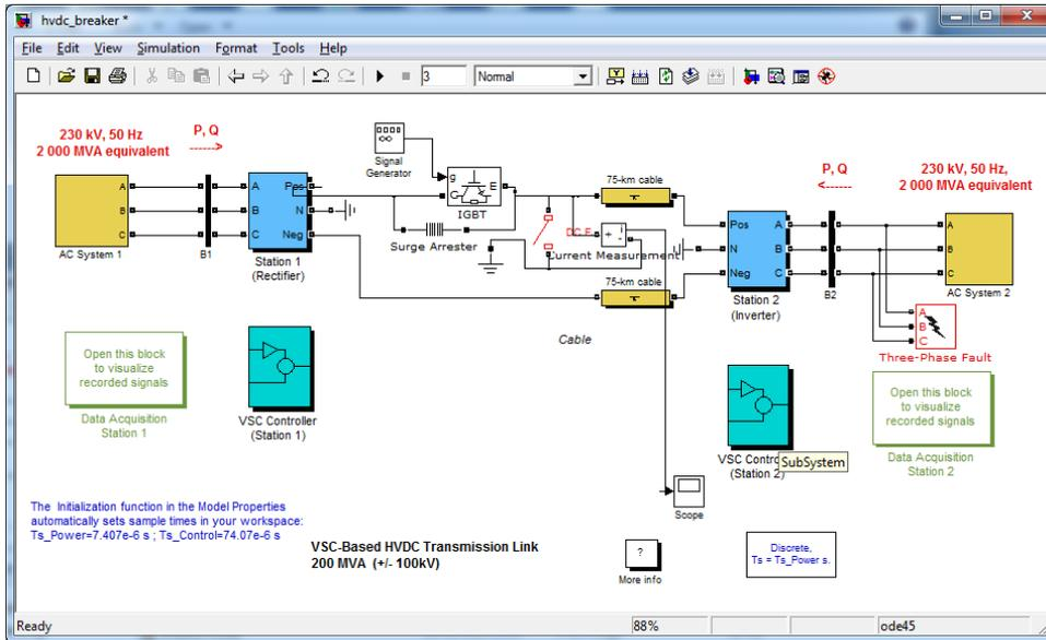
**Figure 7: HVDC MATLAB model**
