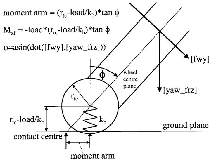
Figure 5. Rounded profile of a typical motorcycle tyre, showing how the overturning moment,  $M_{xf}$ , arises and how it is computed.
