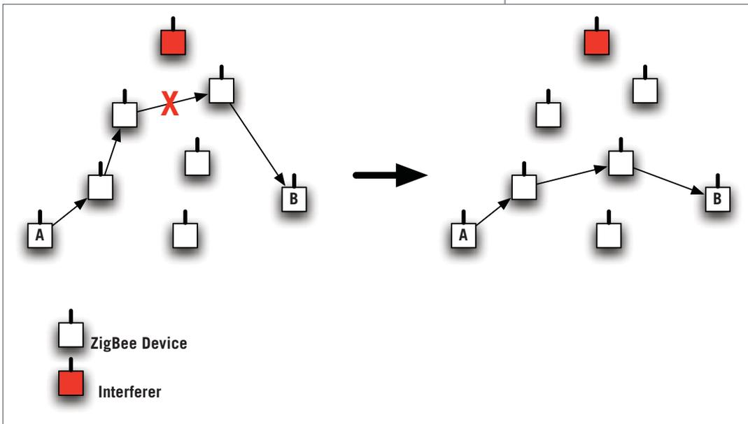
Figure 7 - Mesh Network with Interference
