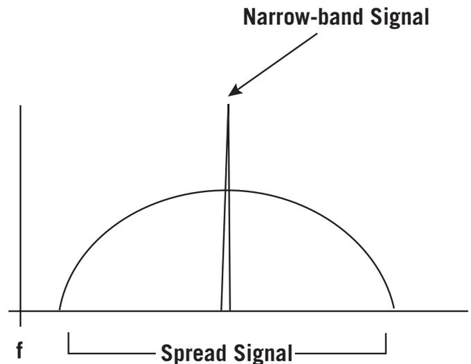
Figure 3 - Spread-Spectrum Signal
