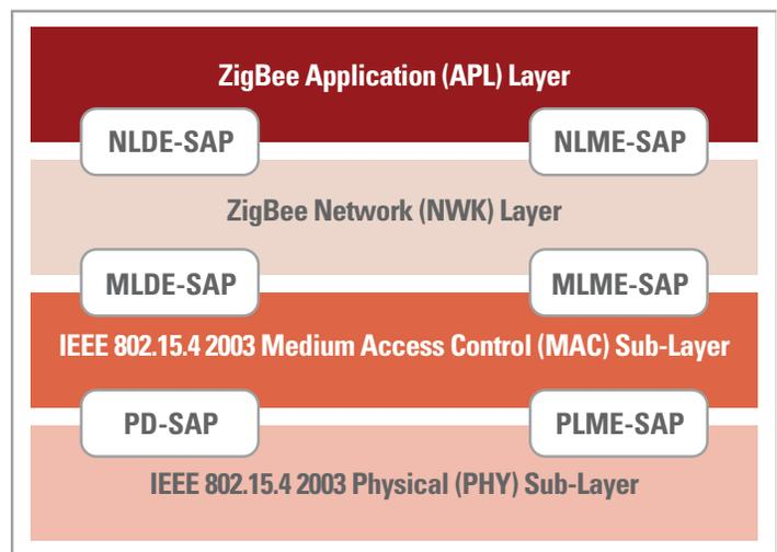
Figure 1 - The ZigBee Stack
