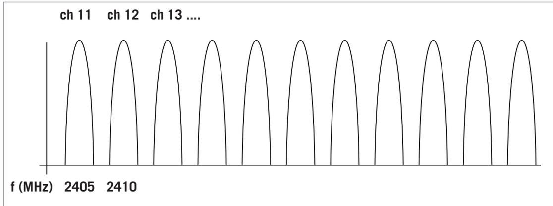
Figure 4 - The 802.15.4 2.4 GHz Spectrum
