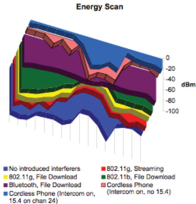
Figure 10 - Interference Sources
