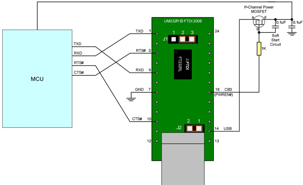
**Figure 6.3 Bus Powered with Power Switching Configuration**
