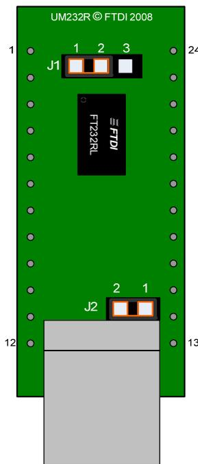
Figure 6.4 USB Bus Powered 3.3V Logic Drive
