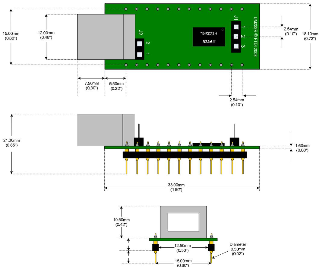
**Figure 4.1 UM232R Module Dimensions**
