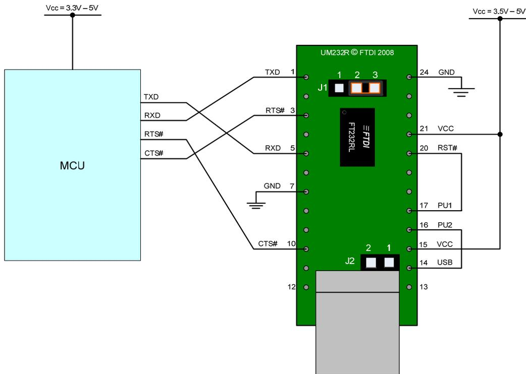
**Figure 6.2 Self-Powered Configuration**
