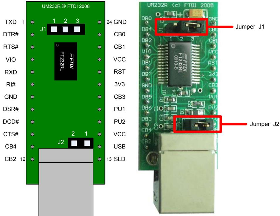
Figure 3.1 Module Pin Out and Jumper Locations
