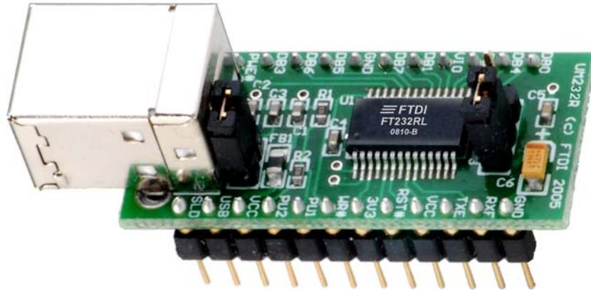
The **UM232R** is a development module which uses FTDI's FT232RL, the one of FTDI's range of USB to UART interface integrated circuit devices.
